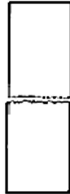
Brittle fracture in steel
