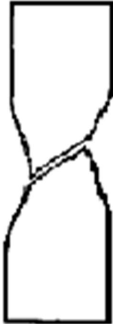
Ductile shear fracture in Aluminum
